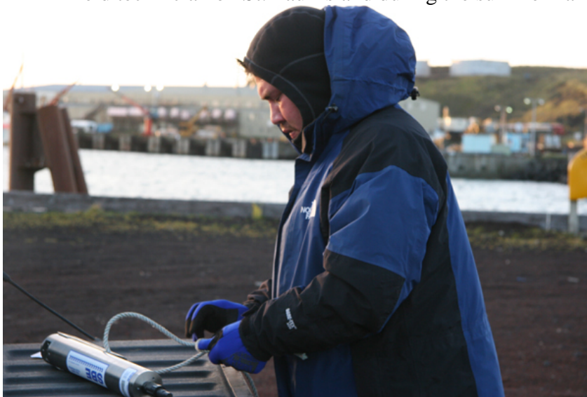
Figure 2. A local researcher prepares a temperature/salinity sensor for deployment in St. Paul harbor for the Pribilof Islands Community-based Ocean Monitoring Program (PICBOMP).
