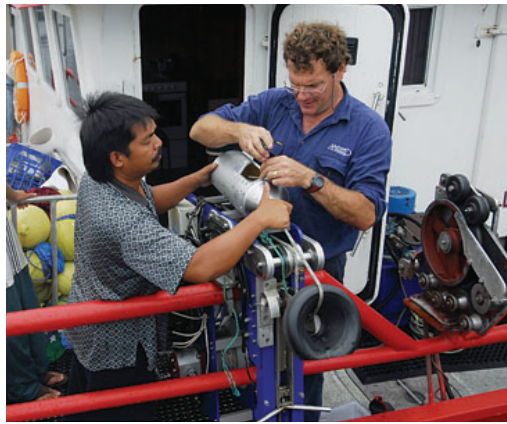
Ian Carlyle of Amerro Engineering works with a deckhand to prepare the prototype underwater setter for testing at sea.
